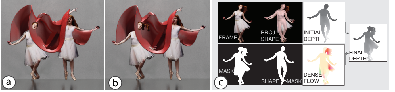
Figure 10. Flow-based refinement. (a) Motion sculpture rendering without refinement; gaps between the human and the sculpture are noticeable. (b) Such artifacts are eliminated with our flow-based refinement scheme. (c) We first compute a dense flow field between the frame silhouette (bottom left) and the projected 3D silhouette (bottom middle). We then use this flow field (bottom right) to warp the initial depth (top right; rendered from the 3D model) and the 3D sculpture to align them with the image contents.
